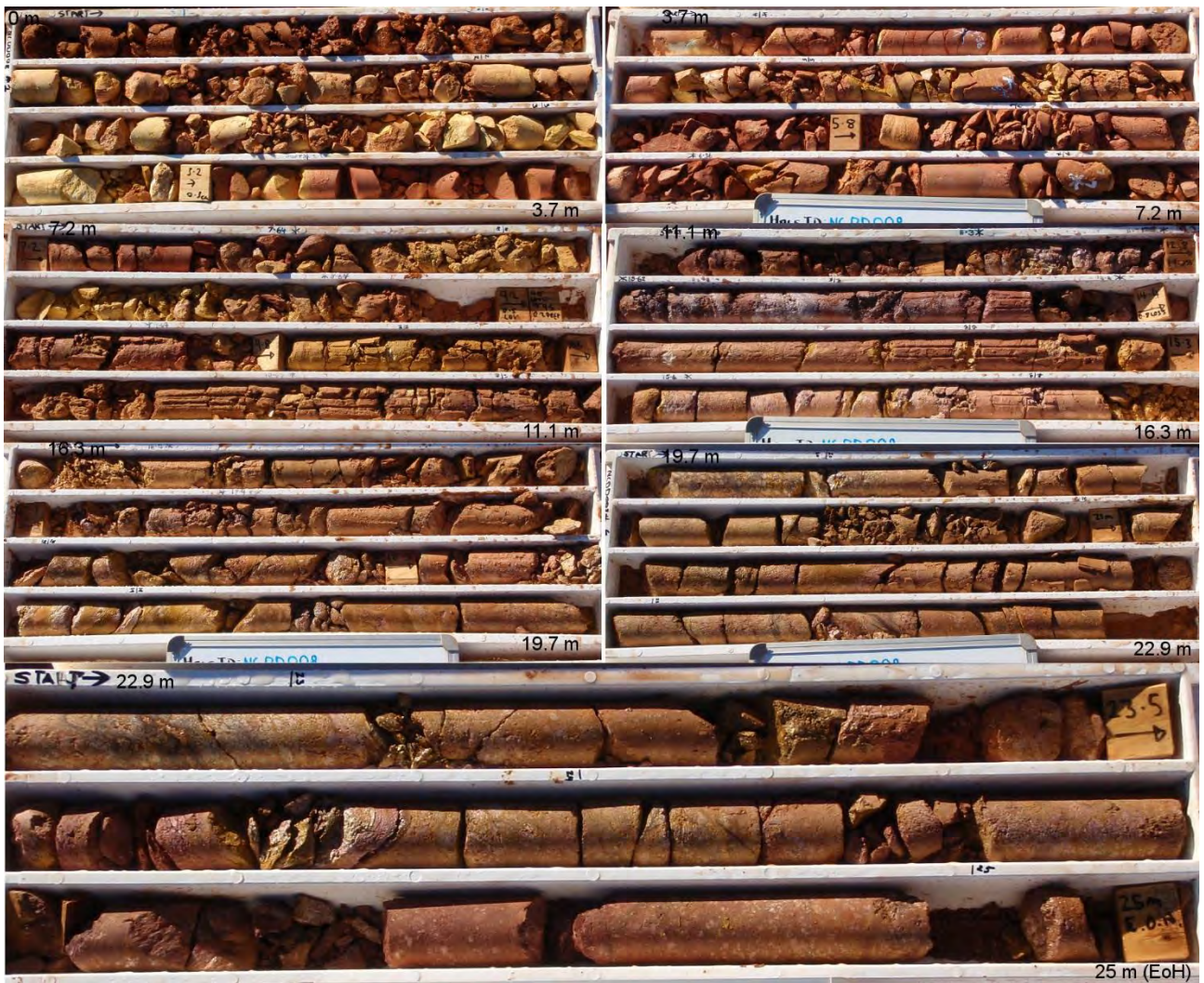
Figure 5-7: Diamond drill core images of Rangoon hole NCDD008 (0 to 25 mbgl) within northern part of proposed Rangoon pit (SWL in area around 20 mbgl).
