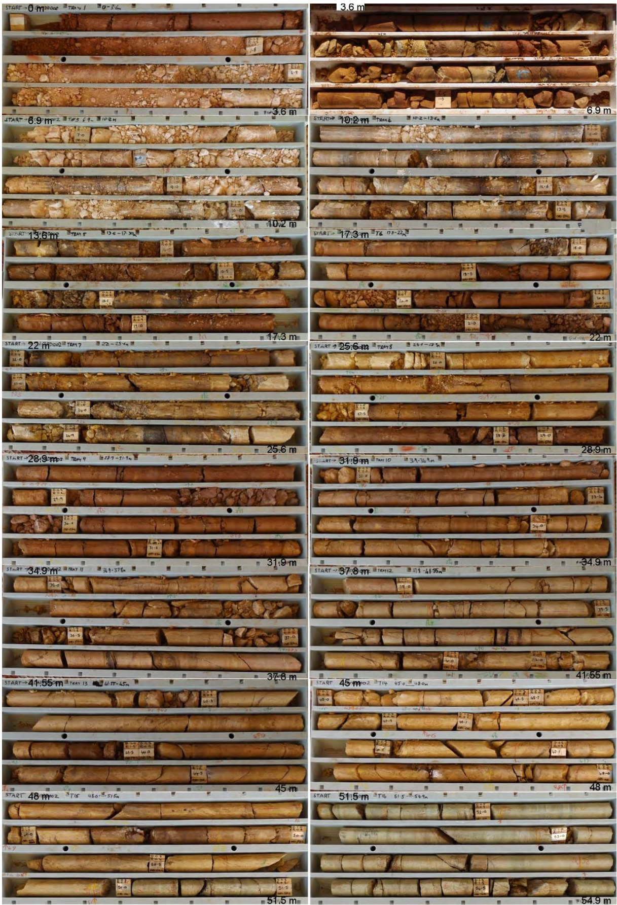
Figure 5-5: Diamond drill core images of Cardinia hole CA17DD002 (0 to 54.9 mbgl) within eastern part of proposed Bruno-Lewis Link pit (SWL in area around 12.7 mbgl).
